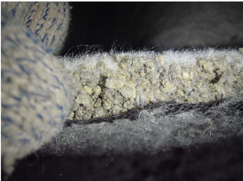
Photo 19: Close-up view of bentonite in a discarded cut portion of GCL liner.
