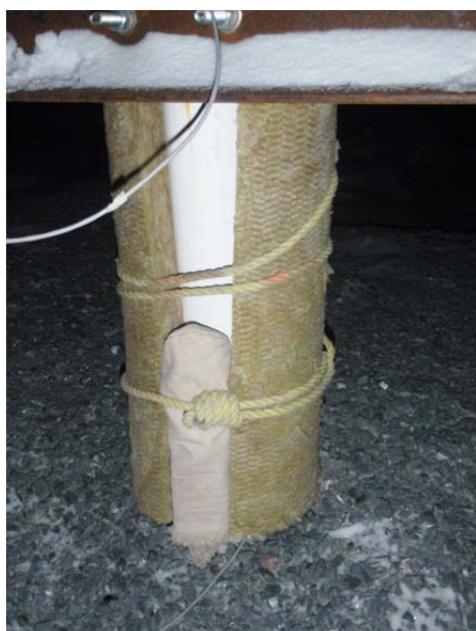
Photo 20: View of thermosyphon performance monitoring test trial. Note that 3" pipe diameter insulation was wrapped around the single bead that was attached to the base of the thermosyphon. Additional testing will result in the coming days
